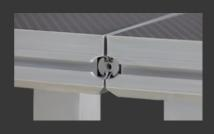
The connection of the platform frames is realised by our quick couplings. The fastening element is made of a specially designed aluminium profile. The frame connector is held securely in place by a specially designed built-in screw so that a very stable connection is created between the frames.
