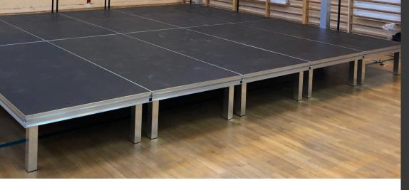
BSC STANDARD is a universal modular stage system recommended for building various types of indoor and outdoor stages, a uditoriums, tribunes/grandstands portable with a height of 0,2 m to 4 m. For structures higher than 1,6 m, additional leg reinforcement is required.
